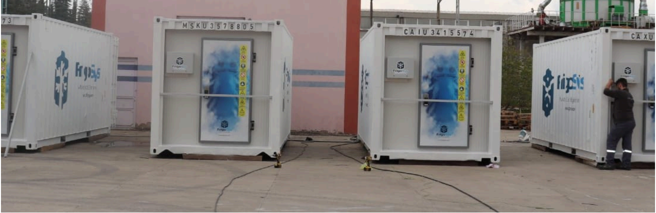
Four 20 ft container cold rooms in final assembly and testing.
